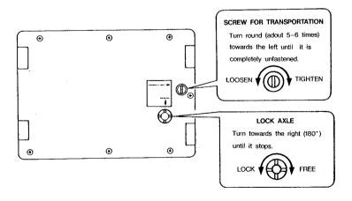
Before plugging the unit in, be sure to loosen the transportation screw and the lock axle on the bottom of the unit with a screw driver.
